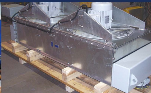
OFAF oil forced, air forced, customized model
